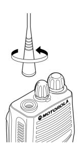
Turn the antenna clockwise to attach it.
